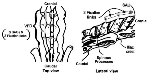
**Fig 2.** External linking system (vertebral fixation device = VFD in illustration on the left) used in this study. Left illustration is a dorsal (top) view and right illustration is a right lateral view. The saddle-shaped SAUs fit over the lower three lumbar spinous processes. (Reprinted with permission from Cramer et al<sup>3</sup> *Journal of Manipulative and Physiological Therapeutics* 2004;27:141-54.)
