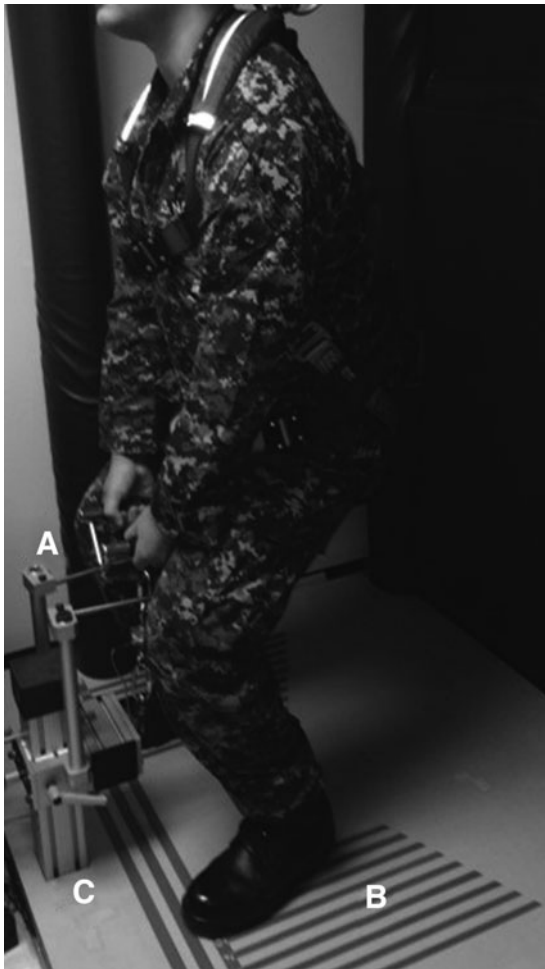
FIG. 1. Strength test: Isometric pulling on a bimanual handle (A) attached to a force transducer. The most comfortable foot position was noted using floor markings (B) and repeated on each test. Handle height was determined by patellar height, set using an adjustable post (C), and remained constant for subsequent tests.
