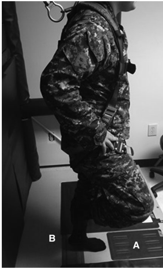
FIG. 2. Balance test: Performed with eyes open and eyes closed. Pressure-sensitive pads (A) were connected to a computer timer. Lifting the heel off pressure-sensitive pad (B) started the timer; once the timer was started, touching any pad with either foot stopped the timer, ending the test.
